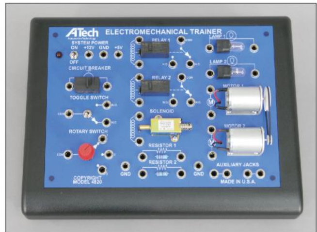
Electromechanical Trainer presents the study of electrical and mechanical circuits. (model 4820)
